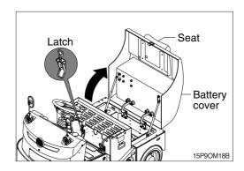
3) Loosen the stopper bolt with hand and remove the battery support.
